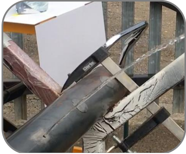
Water leaking out of a steel pipe at 30psi
