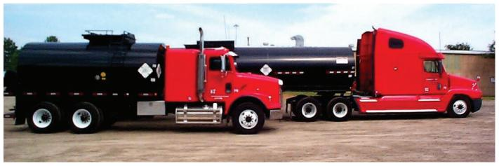
Fill-Coat #1 is delivered to the job site via Trenton's 3000- and 6000-gallon tank trucks that are heated and insulated.
