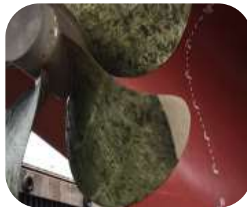
Container vessel propellers suffering from cavitation attack. Surfaces were abrasive blast cleaned and rebuilt using 201 Ceramic Repair Paste
