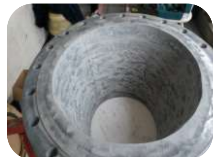
Sea water pipe spool reducer was internally corroded and in need of repair, surfaces were mechanically abraded and rebuilt using 201 Ceramic Repair Paste
