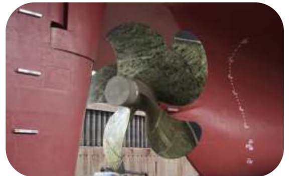
Container vessel propellers suffering from cavitation attack. Surfaces were abrasive blast cleaned and rebuilt using 201 Ceramic Repair Paste
